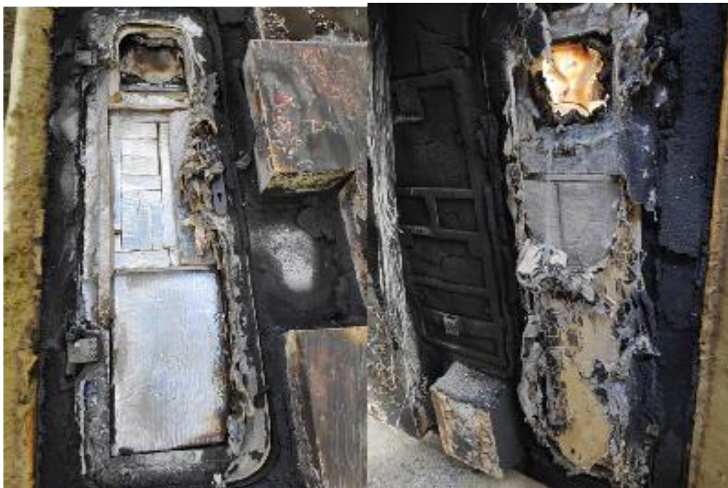
Fig. 8. Doors after the test (exposed side).
