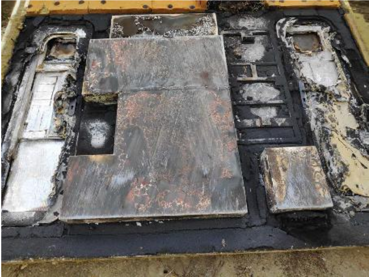
Fig. 7. Test specimen after the test (exposed side).
