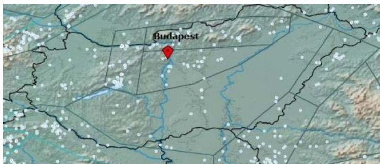
Fig. 1. The localisation of Budapest at 47.49 lat. N/19.03 long. E in decimals - seismic hazard zone polygon delimited, represented on the web platform hazard EFEHR (European Facilities for Earthquake Hazard and Risk). The earthquake data (white circles) are extracted from online ESHM20 Unified earthquake catalogue (Danciu et al., 2021).
